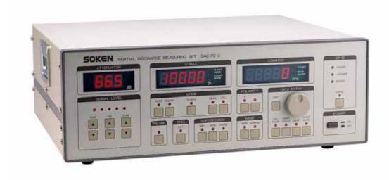
DAC-PD-3 provides Wide Band(10kHz ~ 4MHz) and Narrow Band(10kHz ~ 200kHz). Since bandwidth can be easily chosen in accordance with the kind of specimen, measuring sensitivity, etc., DAC-PD-3 is available for partial discharge test such as electric equipments, electronic parts and insulating materials.
